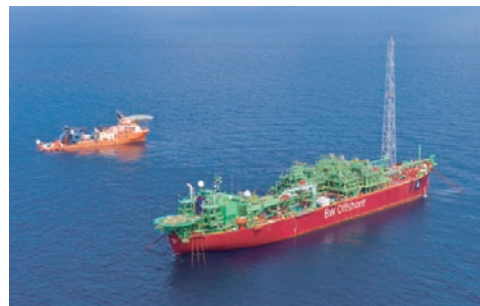
Floating Production Unit (FPU) located at Terang Gas Field, Kangean PSC
