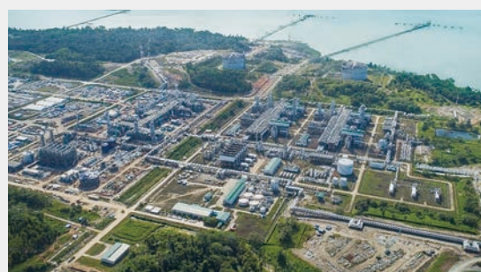
Liquefaction plant existing second system and expanded system under construction, LNG tanks, jetty, etc.
