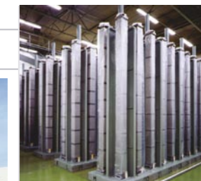
Nuclear fuel assemblies for PWRs. Approx. 4 meters in length.
