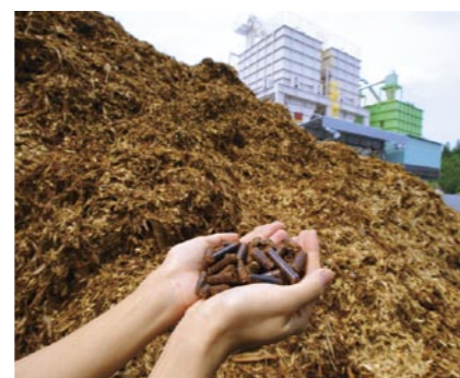
Bio-pellets (wood pellets) are a solid fuel made from materials such as bark.
